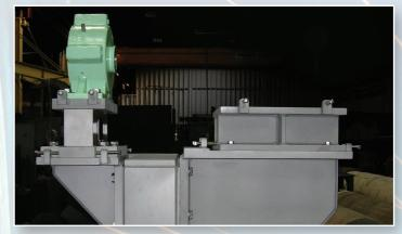
Framework Support Section Engineered for Increased Loading
